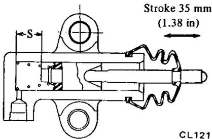
Fig. CL-16 Non-adjustable operating cylinder
