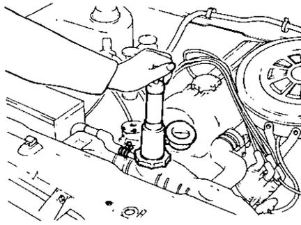
Fig. CO-11 Testing radiator
