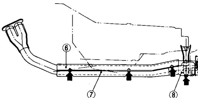
Fig. FE-14 Exhaust front tube heat shield plate
