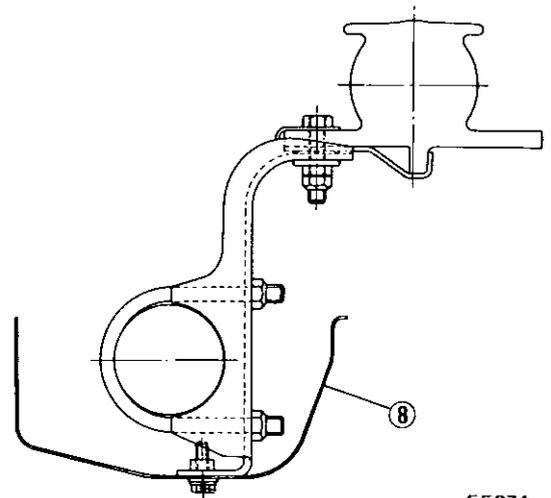
Fig. FE-15 Exhaust front tube mounting bracket
