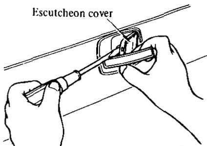
Fig. BF-42 Removing escutcheon cover
