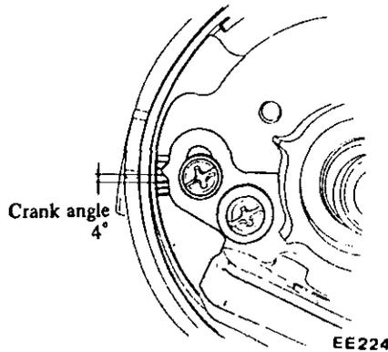
Fig. ET-34 Phase difference adjusting scale
