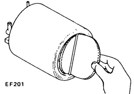
Fig. ET-49 Replacing carbon canister filter
