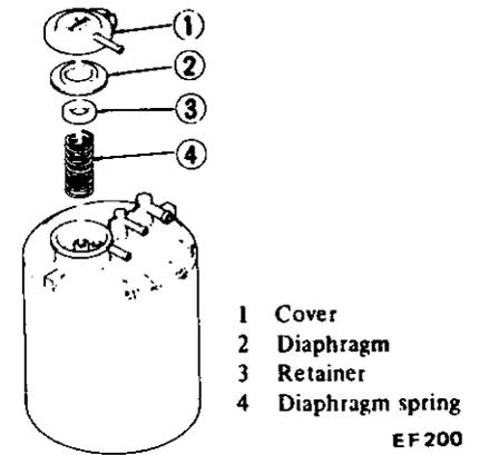
Fig. ET-48 Carbon canister purge control valve
